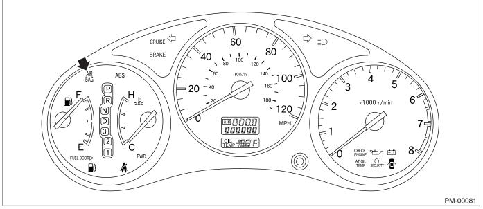
2) Turn the ignition switch to ON, and connect the airbag diagnosis terminal of the service connector (located below lower cover) to ground terminal.
