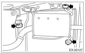
3) Remove the front, right and left cushion rubber, and detach the muffler assembly.
