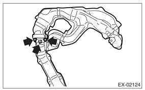
10) Remove the front oxygen (A/F) sensor and the rear oxygen sensor. <Ref. to FU(H4SO)-36, RE-MOVAL, Front Oxygen (A/F) Sensor.> <Ref. to FU(H4SO)-37, REMOVAL, Rear Oxygen Sensor.>
