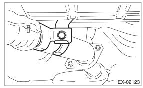
8) Remove the front and center exhaust pipe assembly from vehicle.
