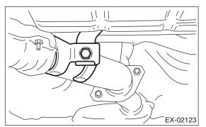
5) Tighten the nuts which hold the front exhaust pipe onto cylinder heads.
