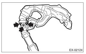
3) Install the front and center exhaust pipe assembly to vehicle.
