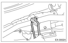
3) Apply a coat of spray type lubricant to the mating area of cushion rubbers in advance.
