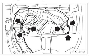
7) Remove the bolt which installs the front and center exhaust pipe assembly to hanger bracket.
