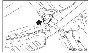
3) Install the rear exhaust pipe to muffler.
