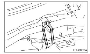
4) Install the rear exhaust pipe to center exhaust pipe.
