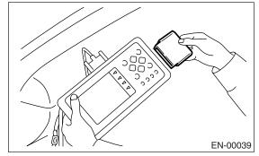
4) Connect the Subaru Select Monitor to data link connector.
