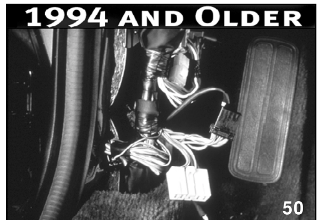
Select Monitor and Service Connector
