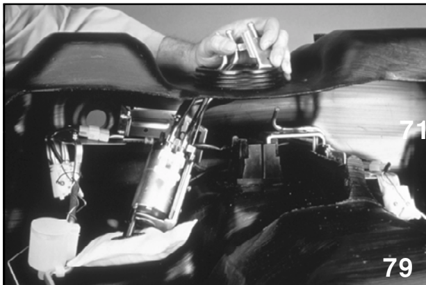
Removing Fuel Pump
