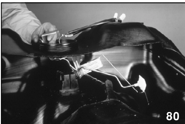
Removing Sending Unit
