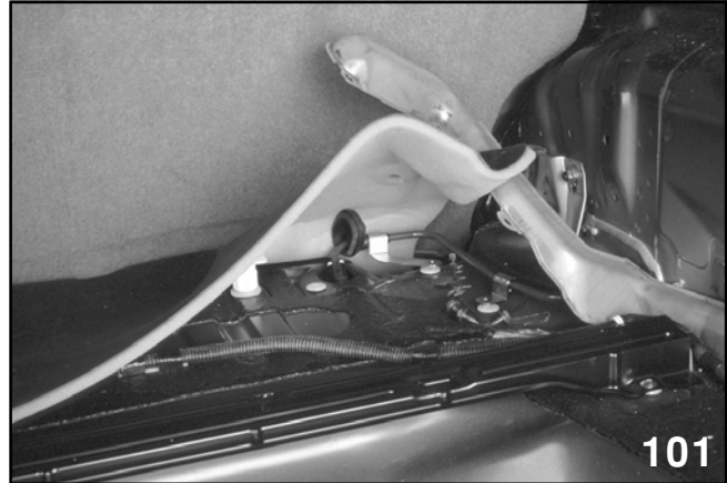
Vent Control Piping
