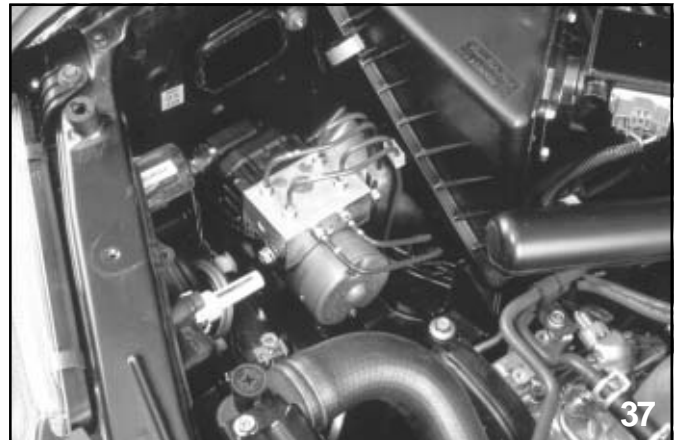
Hydraulic control unit
