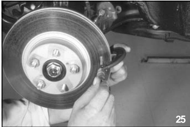
Measuring rotor thickness
