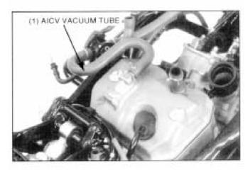
Remove the cylinder head cover bolts, washers and rubber seals.
