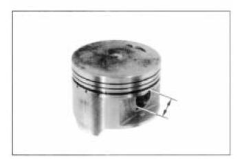
Measure the piston pin O. D. at three points.
