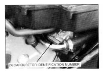
(3) The carburetor identification numbers are stamped on the intake side of the carburetor body as shown.
