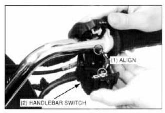
Install and tighten the screw.
