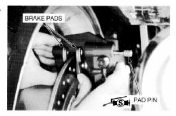
Tighten the pad pin to the specified torque.
