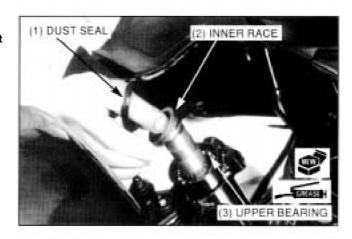
Apply oil to the steering top threads.
