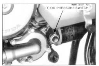
Start the engine and check the oil pressure at 6,000 min<sup>-1</sup> (rpm)
