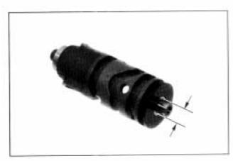
Install the dowel pins into the cam plate holes.
