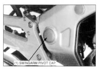
Loosen and remove the left pivot lock nut using the special tool.
