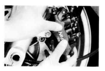
Remove the pad pin plug and pad pin.
