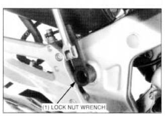
Loosen the swingarm adjusting bolt by turning the pivot bolt.
