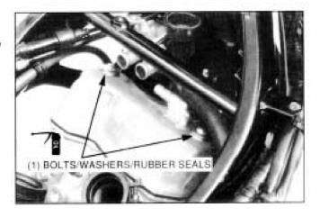
Install the thermostat housing to the frame. Install and tighten the mounting bolt.
