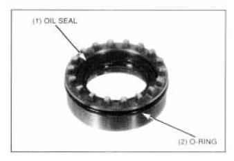
Driver a new oil seal into the retainer using the special tools.
