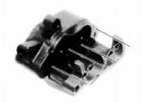
Check the caliper piston for scratches, scoring or other damage.
