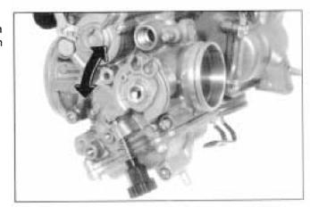
Turn the throttle stop control knob to align the rear cylinder carburetor throttle valve with the edge of the by-pass hole.
