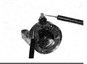
Check for continuity between each commutator bar and the armature shaft. There should be no continuity.
