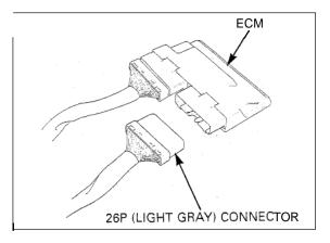
Connect the peak voltage tester or peak voltage adaptor probes to the connector terminal of the wire harness side and ground.
