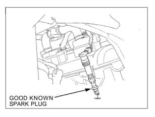
With the ignition coil sub-harness 4P (Black) connector connected, connect the peak voltage adaptor or Imrie tester to the 4P (Black) connector primary wire terminal and ground.
