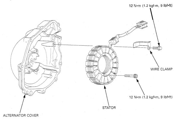
Install the stator into the alternator cover.
