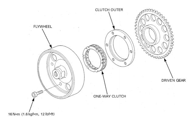
Apply oil to the starter one-way clutch. Install the one-way clutch into the clutch outer with the flange side facing out.
