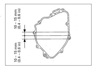
Install the dowel pin and new gasket.
