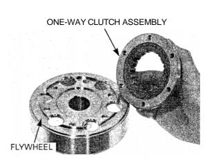
Apply a locking agent to the starter clutch outer mounting bolt threads.
