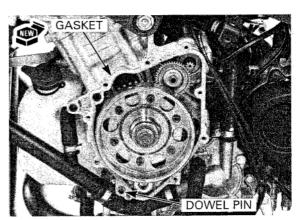
The aitemator cover (stator)is magnetically attached to the flywheel, be careful during installaInstall the alternator cover.
