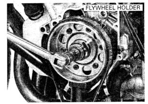
Remove the flywheel using the special tool.
