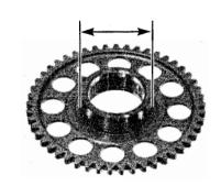
Check the one-way clutch for wear or damage and replace if necessary.
