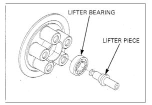
Install the lifter bearing into the pressure plate. Install the clutch lifter piece into the lifter bearing.
