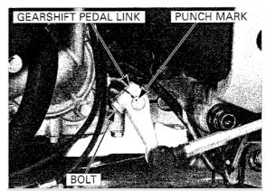
Install the gearshift pedal link aligning its slit with the punch mark on the gearshift spindle.
