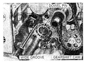
Apply a I cking gent o the gearshift cam socket bolt threads.
