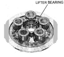
**Clutch spring** Measure the clutch spring free length.
