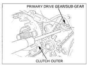
Remove the oil pump driven sprocket bolt/washer. Remove the oil pump drive/driven sprocket and drive chain as an assembly.
