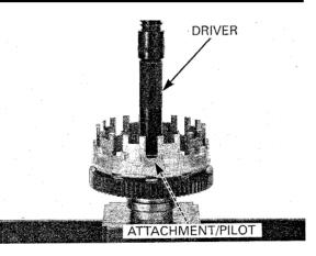
Press the needle bearing into the clutch outer with the marked side facing up Press a new needle bearing into the clutch outer so that the casing of the needle bearing is flush with the clutch outer surface as shown.
