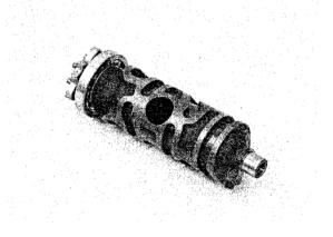
Turn the outer race of the shift drum bearing with your finger.
