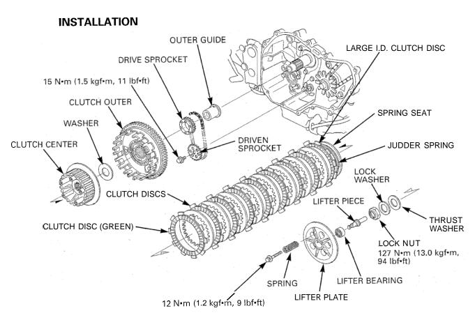
install the oil pump driven sprocket with its "OUT" mark facing out Install the clutch outer guide, and then install the oil pump drive/driven sprocket and drive chain as an assembly.
