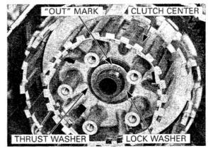
Apply oil to the new lock nut threads, then install it.
