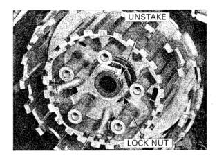
Hold the clutch center with the clutch center holder, then remove the lock nut.
