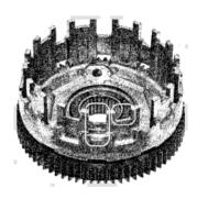
Measure the O.D. and I.D. of the clutch outer guide.
