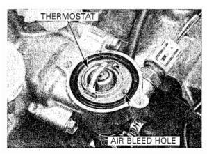
Install the thermostat housing cover onto the housing.
