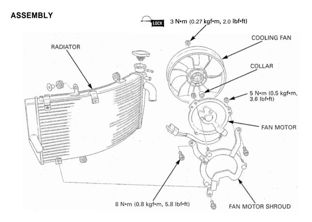
Install the fan motor onto the fan motor shroud with the drain hose facing as shown.
