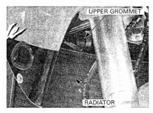
Install the washer and upper mounting bolt, then tighten the bolt.
