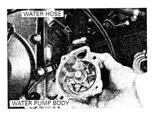
Apply engine oil to a new O-ring and install it onto the stepped portion of the water pump.
