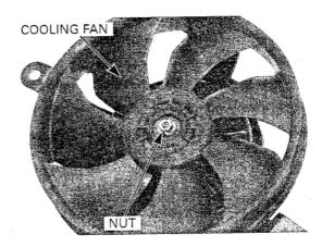
Remove the flange nuts and fan motor from the fan motor shroud.
