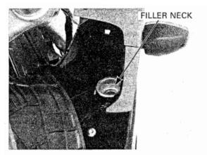
Remove the radiator reserve tank cap and fill the reserve tank to the upper level line.
