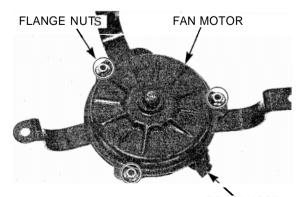
Install the distance collar onto the fan motor shaft. Install the cooling fan onto the fan motor shaft by aligning the flat surfaces.
