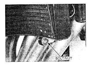
Remove the radiator upper mounting bolt and washer.
