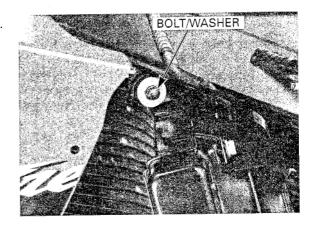
Be careful not to damage the radiator core Slide the radiator to the right, then release the upper grommet from the frame boss. Remove the radiator assembly.
