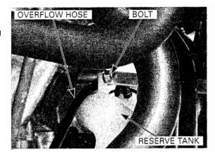
Install and tighten the lower mounting bolt. Connect the siphon hose to the reserve tank
