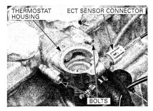
Disconnect the fast idle wax unit water hose and bypass hoses from the thermostat housing.
