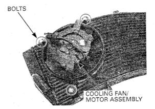
Remove the nut, cooling fan and distance collar.
