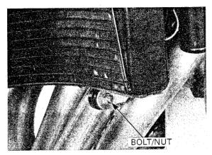
Connect the fan motor **2P** (Black) connector. Connect the lower radiator hose and tighten the clamp screw securely.
