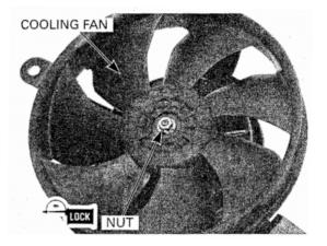
Install the cooling fan/motor assembly onto the radiator. Install and tighten the bolts to the specified torque.
