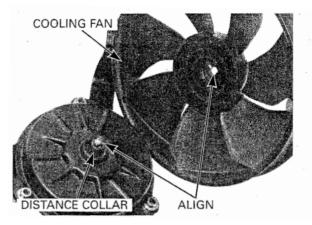
Apply a locking agent to the cooling fan nut threads. Install and tighten the nut to the specified torque.
