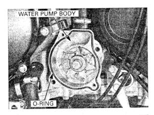
Disconnect the water pump-to-water joint hose from the water pump body.
