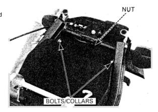
Unhook the rear fender from the seat rail brace, then release the regulator/rectifier wire and main wire harness from the seat rail and rear fender.
