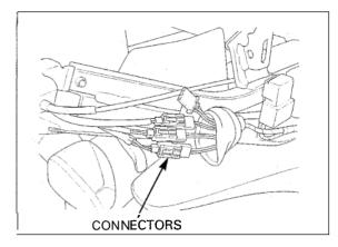
Remove the headlight relay, engine stop relay and fan control relay from the rear fender.
