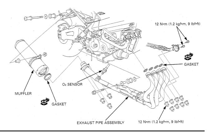
Install the exhaust pipe mounting rubber and collar into the lower bracket hole.
