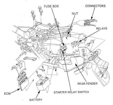
Install the rear fender aligning its lower groove with the seat rail brace.
