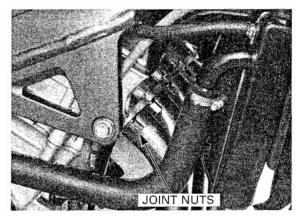
Temporarily tighten the exhaust pipe mounting nut.
