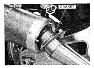
Temporarily install the muffler mounting bolt/nut and muffler joint nuts.
