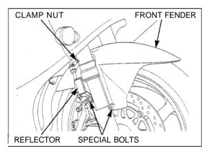
Remove the front fender by pulling it forward.
