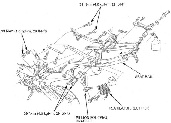
Install the seat rail and tighten the mounting bolls and nuts to the specified torque.
