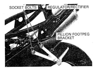
Install the right pillion footpeg bracket and tighten the socket bolts to the specified torque.
