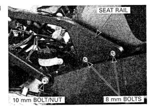
Install the regulator/rectifier, tighten the bolts.
