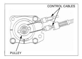
Install the EGCV pulley cover and tighten the bolts to the specified torque.
