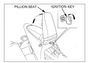
Remove the pillion seat mounting nuts, then remove the seat belt and pillion seat.
