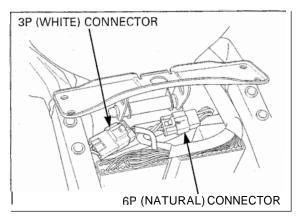
Disconnect the turn signal connectors and license light connector.
