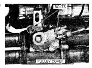
Disconnect the EGCV control cables from the pulley.
