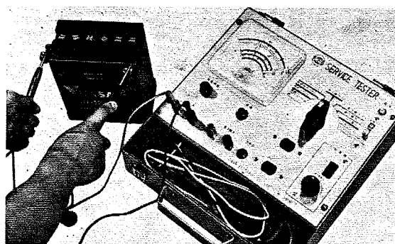
Fig. 5-96. D.C. voltage measurement
