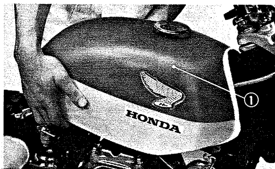
① Fuel tank Fig. 4-34. Installing the fuel tank
