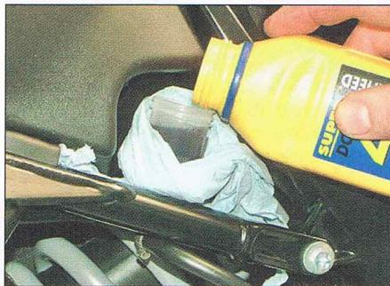
**4** Top-up with new DOT 4 brake fluid, until the level is just below the MAX level line. Do not overfill and take care to avoid spills.
