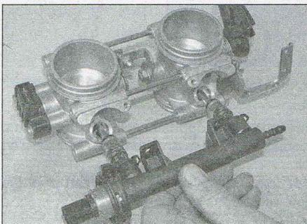
10.4a Lift the fuel rail assembly off the throttle bodies
