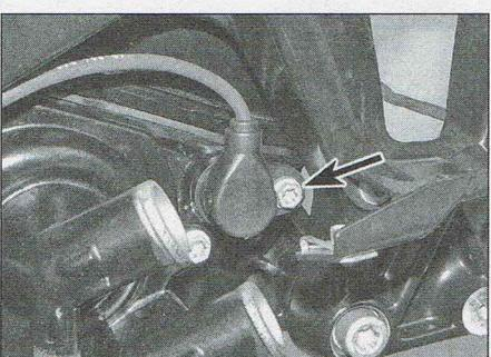
17.14a Undo the screw securing the camshaft position sensor...
