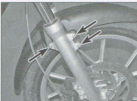
2.30 Screws secure front mudguard on both sides
