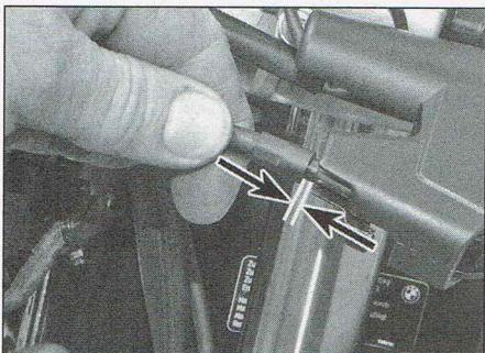
4.3 Measure the gap (arrowed)
