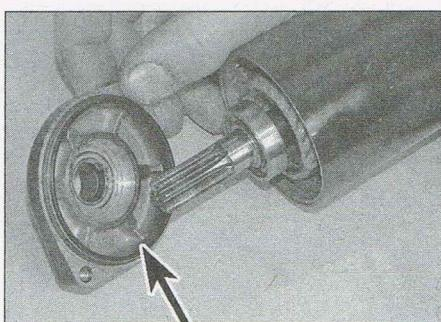
22.9b ...and remove the front cover – note the sealing ring (arrowed)
