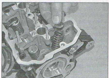
11.11a Remove the spring retainer...
