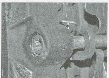
2.23b Spring clip correctly located in pad pin groove
