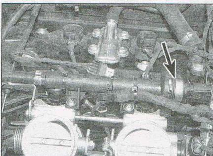
7.1 Location of the fuel pressure sensor (arrowed)
