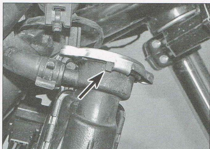
15.11 Tighten the radiator cap against the stop (arrowed)
