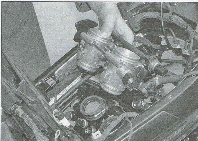
9.9 Ease the throttle body assembly out of the adapters
