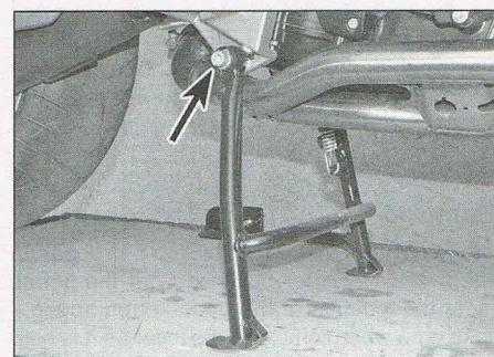
4.14b Remove the pivot bolts on both sides
