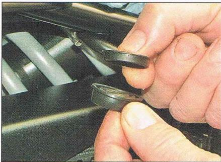
**3** ... and remove the diaphragm plate and diaphragm.
