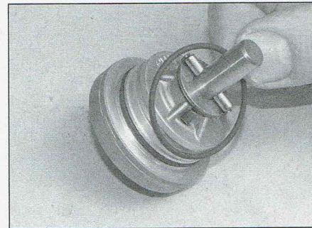
8.12 Remove the pump body O-rings
