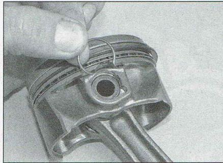
24.19 Align the circlip to aid installation
