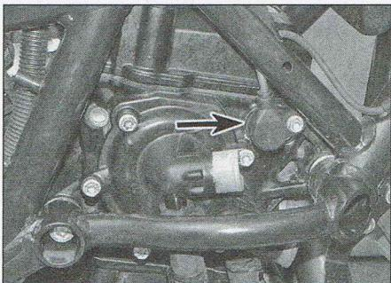
17.9a Location of the camshaft position sensor – GS models
