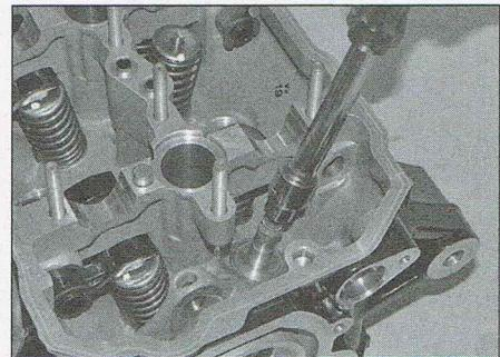
11.32 Press the seal into place with a suitable deep socket
