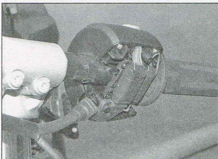
5.10c Disconnect the wiring connectors
