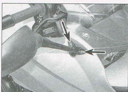
4.40a Undo the screws (arrowed)...
