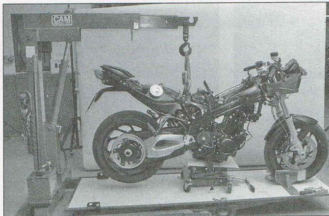
4.23 Set-up for supporting the engine and the frame
