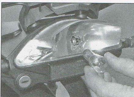
8.4 Line up the pins on the bulb with the slots in the socket
