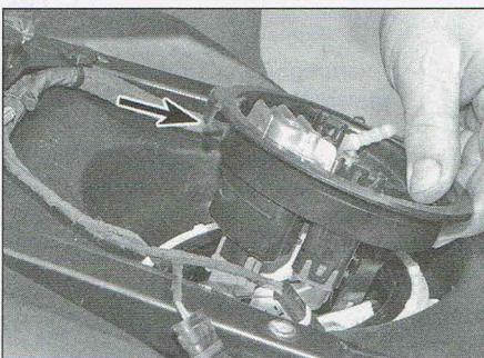
5.9b ...noting the locating tab (arrowed)
