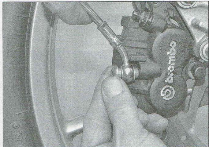
3.3b Sealing washers are fitted both sides of the union
