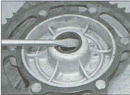
17.45 Levering out the coupling bearing seal
