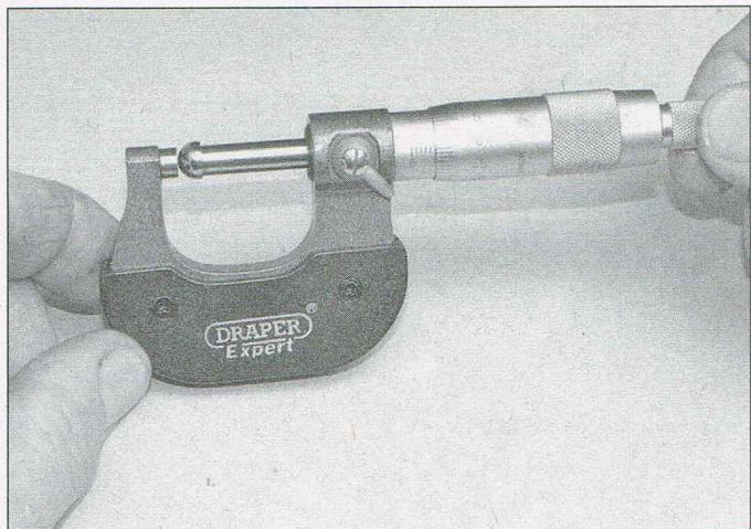
10.11b Measuring the shim with a micrometer
