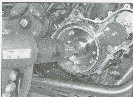
24.13a Heat the rotor bolt to soften the locking compound
