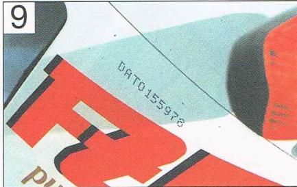
Chemically-etched code numbers can be applied to main body panels . . .
