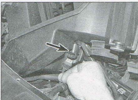
2.17 Disconnect the idle actuator wiring connector
