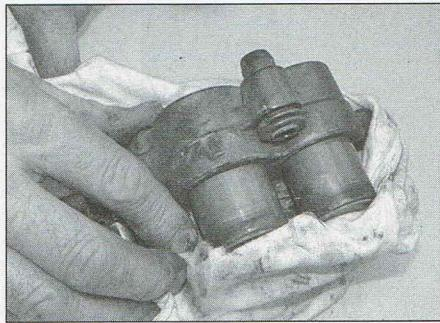
3.15b ...until the pistons are displaced
