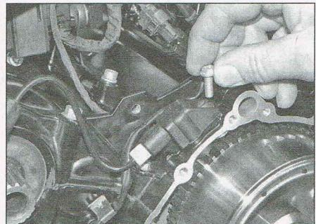
17.5a Undo the screw securing the ignition timing sensor...
