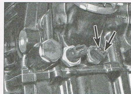
4.5 Measure resistance between the sensor terminals
