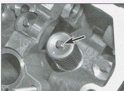
11.34 Installed position of the valve collets
