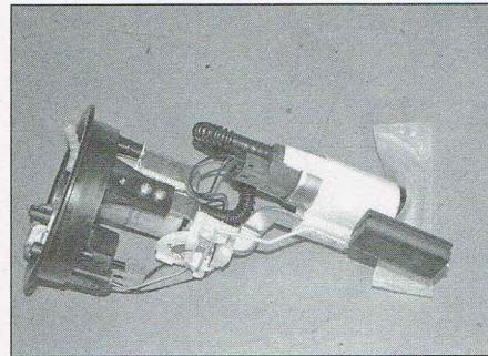
5.10e Inspect the wiring and terminals for damage
