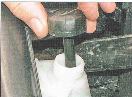
**2** If the coolant level is on or below the MIN line, remove the reservoir filler cap.
