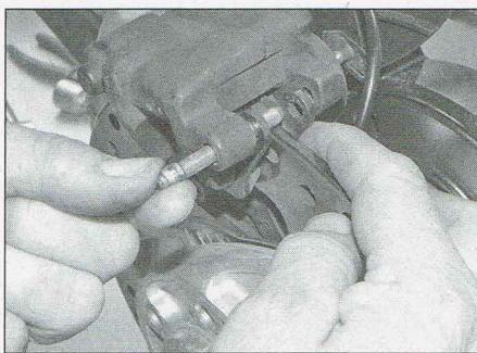
6.18a Align the holes in the pad and caliper...
