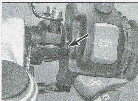
5.14 Alignment mark on switch housing (arrowed)
