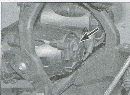
**6.2a Headlight high beam bulb housing**
