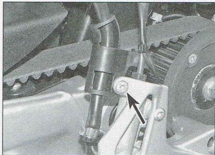
9.11a Screw (arrowed) secures brake hose guide
