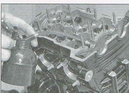
8.30 Lubricate the bearing surfaces with engine oil
