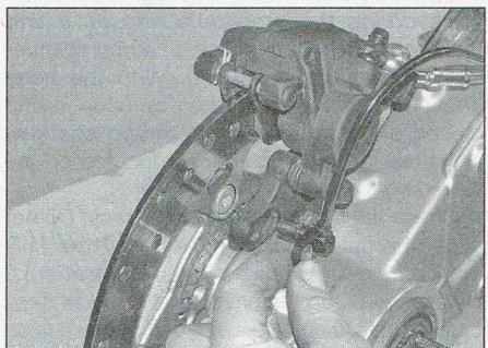
10.10d ...and remove the speed sensor – S, ST and GT models
