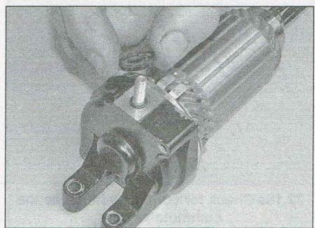
22.11b ...remove the insulating washer...
