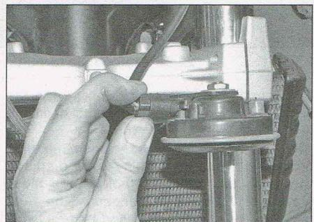
20.5 Check the horn connector and terminals
