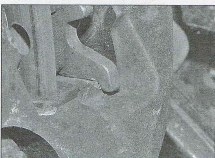
2.22 Locate the tab of the pad backing plate against the caliper (inner pad shown)
