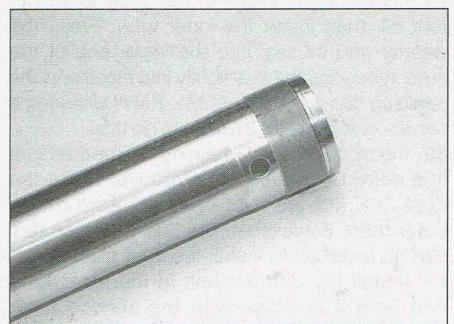
8.70b ...then install the top bush in its groove
