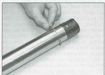
8.67 Slide on the oil seal retaining clip
