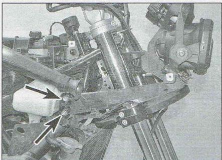
7.5b Undo the screws (arrowed) on both sides...
