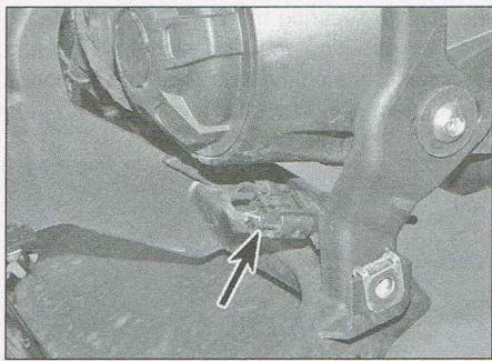
7.5a Location of the air temperature sensor wiring connector
