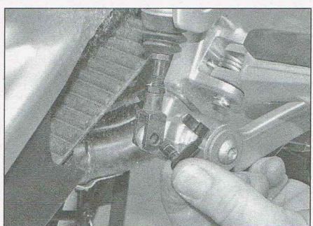
3.8b Release the clip and withdraw the clevis pin
