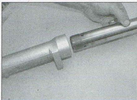
8.22 Slide the inner tube into the outer tube
