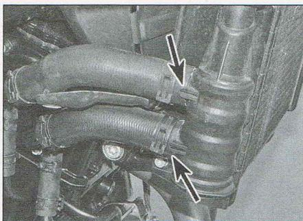
6.5a Note how the cut-outs (arrowed) align with the radiator unions
