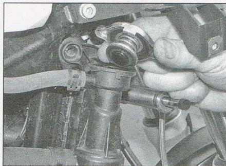
15.8b ...then press down and twist to remove it
