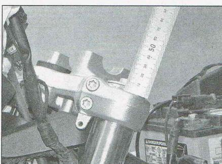
6.8a Measuring fork tube installation – 2009 to 2014 R models
