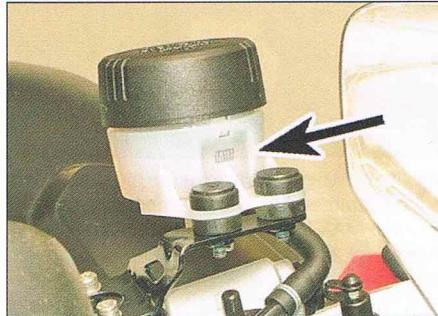
**1** The front brake fluid level is visible through the window in the reservoir body – it must be above the MIN level line.
