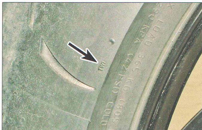
**4** Tyre tread wear indicator location marking (arrowed).
