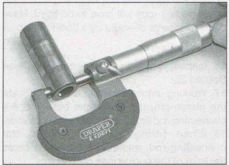
24.14a Measure the piston pin at each end...
