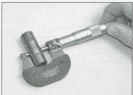
24.14b ...and in the centre to check for uneven wear
