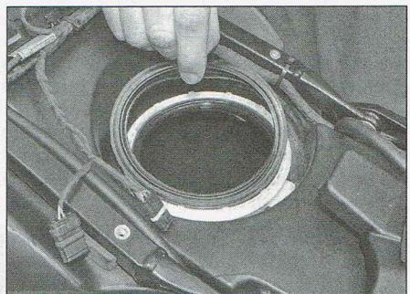
5.9c Fit a new pump seal on installation
