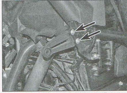
6.11b Undo the screws (arrowed) and remove the bracket
