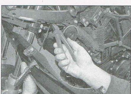
2.14e ...cut any wiring ties...
