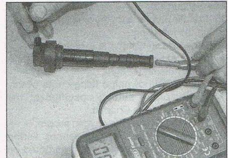
14.7c Measuring the coil secondary resistance
