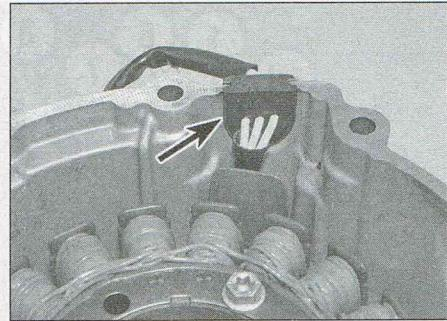
24.20b ...noting the location of the wiring grommet
