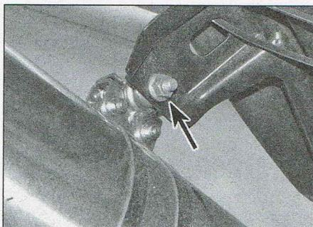
11.2b ...and unscrew the nut on the inside of the bracket
