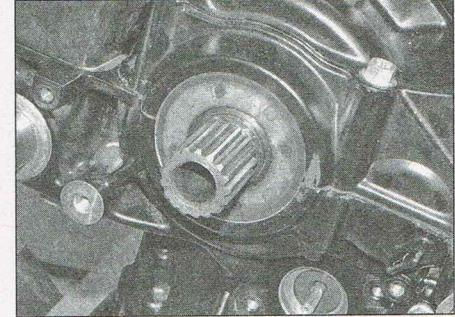
26.15b Installed position of the output shaft seal
