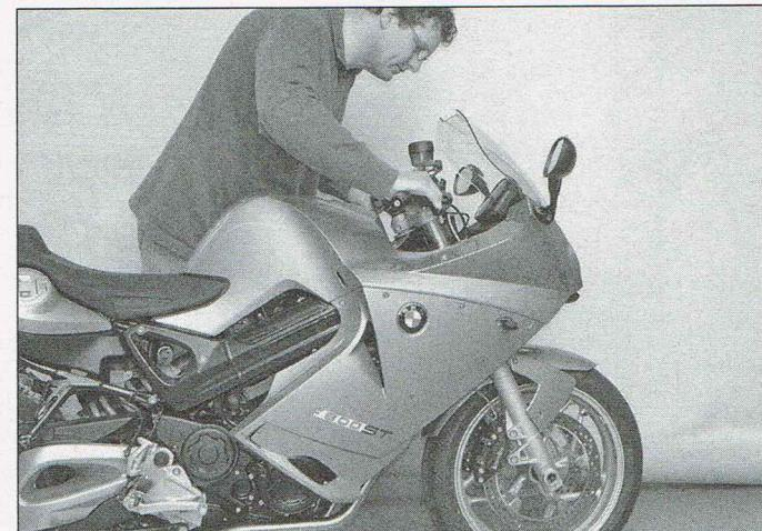
13.2 Checking the action of the front suspension
