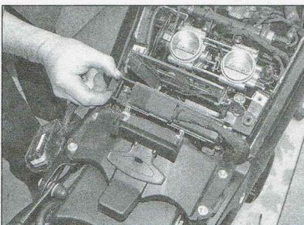
16.7a Disconnect the engine wiring harness connector...
