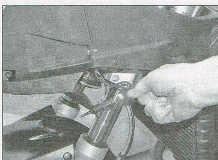
7.16 Disconnect the air temperature sensor wiring connector
