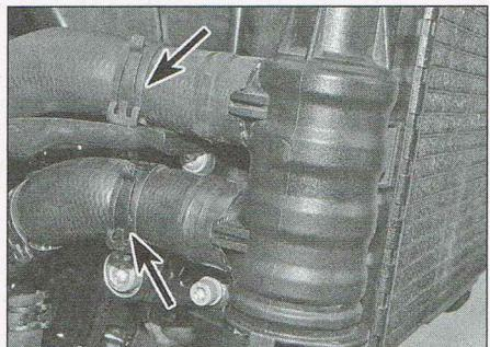
9.2b ...to slide the hose clips (arrowed) off the unions
