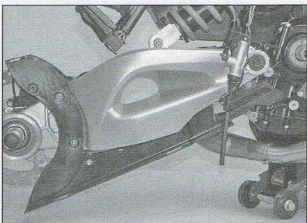
13.10a Remove the rear section of the belt guard...
