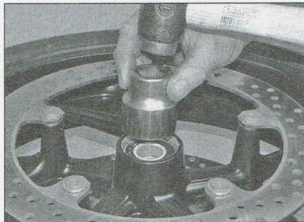
17.11 Using a socket to drive the bearing in
