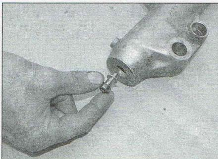
8.27 Fit a new sealing washer onto the damper bolt
