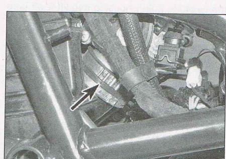
**9.8b** Throttle body clamp (arrowed) – F650 GS model shown
