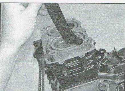
9.13b ...and lift out the tensioner blade
