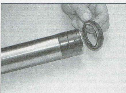
8.66 Install the dust seal ensuring it is the correct way round
