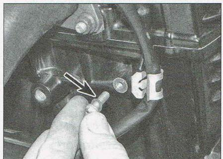
2.15 Fit a new sealing washer to the drain bolt
