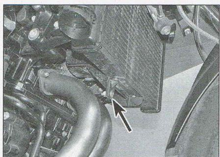
6.8a Undo the screw and nut...
