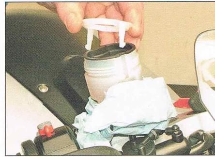
**6** Ensure that the diaphragm is correctly seated before installing the diaphragm plate and cover. Tighten the cap securely.
