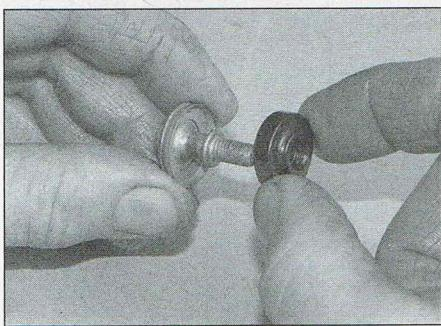
6.11c ...noting how the sealing washers fit
