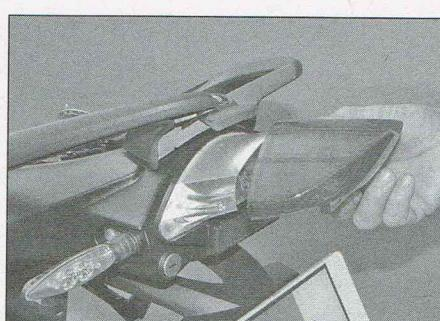
8.1b ...and remove the lens
