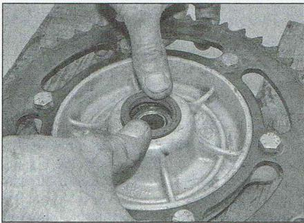
17.50c Press in the new bearing seal
