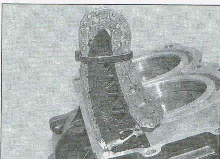
10.6b Cam chain is secured with a cable-tie
