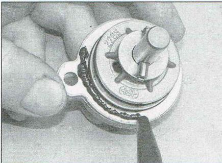
8.19 Apply a thin coating of sealant
