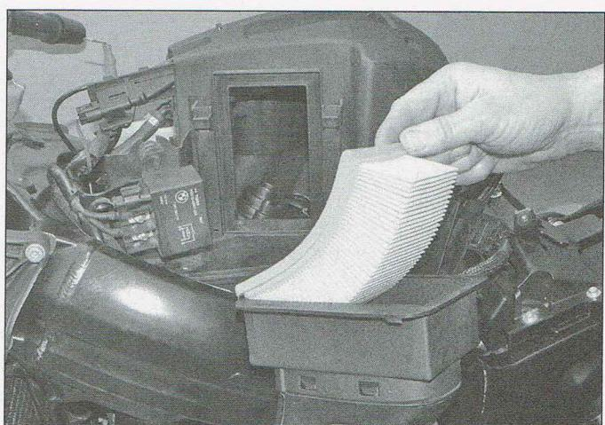
11.3c ...and lift out the filter element
