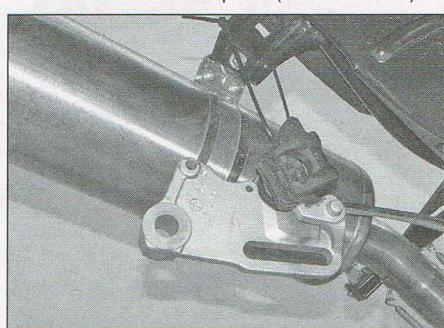
7.1b Secure the caliper bracket to avoid straining the brake hose
