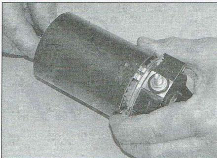
22.10a Ease the armature out through the main housing...
