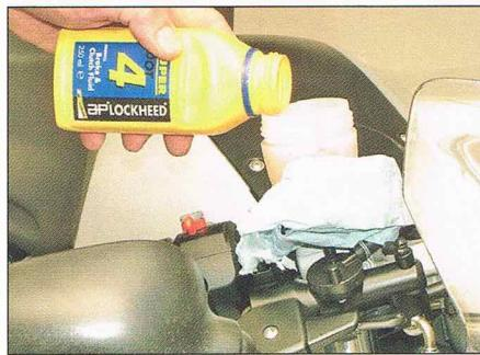
**4** Top-up with new DOT 4 brake fluid, until the level is just below the MAX level line. Do not overfill and take care to avoid spills (see **Warning** above).
