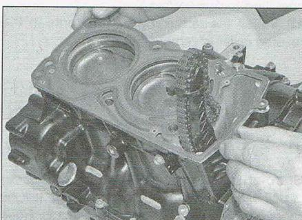
10.6a Remove the cylinder head gasket
