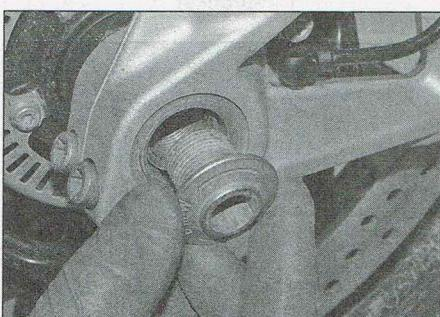
15.7a Slacken the two clamp bolts, then remove the axle bolt from the left side of the wheel...
