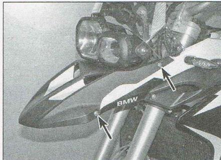
3.11 Screws on both sides secure the upper front mudguard
