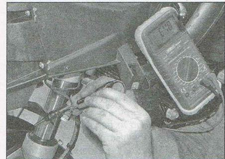
14.5 Measuring the air temperature sensor resistance
