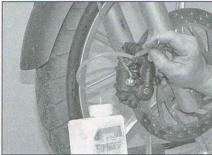
12.2a Set up for bleeding the front brake
