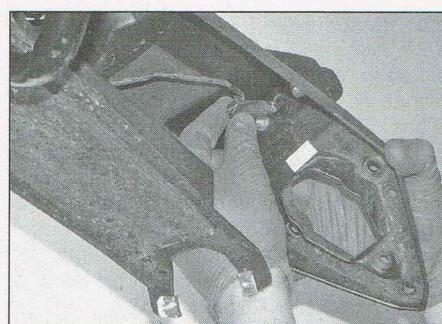
3.30a Pull out the bulb socket
