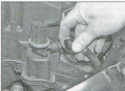
2.15c Disconnect the secondary air system valve hose
