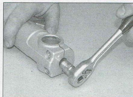
8.2 Loosen the damper bolt
