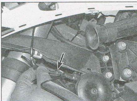
3.12 Free the turn signal wiring
