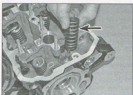
11.11b ...the valve spring, noting the paint marks (arrowed)...
