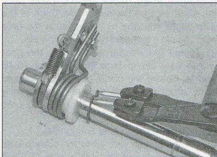
17.6c Slide the circlip along the shaft
