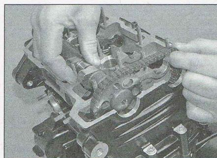
8.6b ...and then the exhaust camshaft
