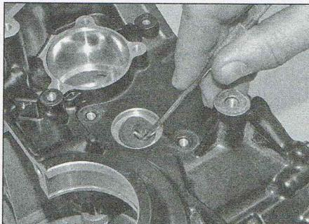
28.13a Removing the seal with a seal hook
