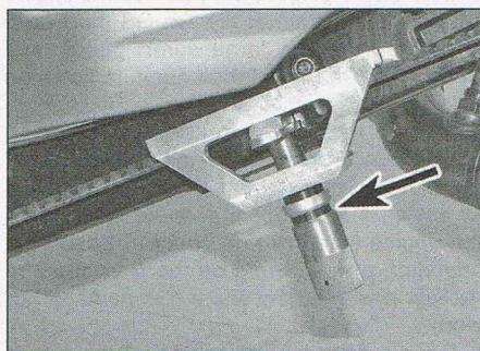
2.8 Read the scale against the upper reference edge (arrowed)
