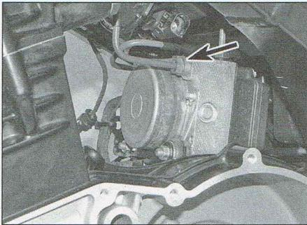
11.4b Gland nut (arrowed) on ABS modulator
