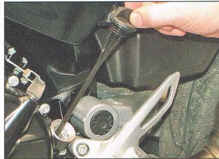
**2** Unscrew the filler cap, withdraw the dipstick and wipe it clean – S, ST, GT and R models shown.
