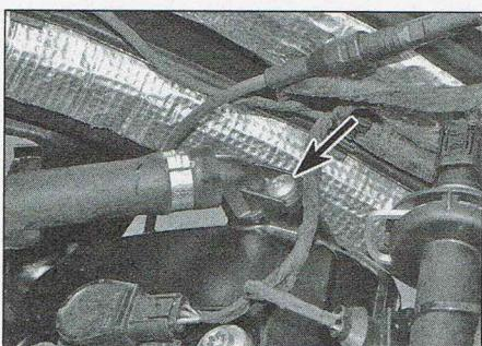
6.8a Undo the screw (arrowed)...
