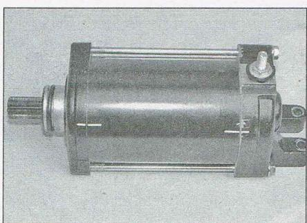
22.8 Make alignment marks between the main housing and the covers
