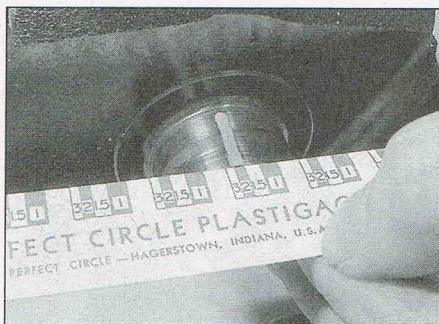
22.20 Compare the width of the crushed Plastigauge with the scale
