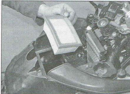
11.2c ...and lift out the filter element
