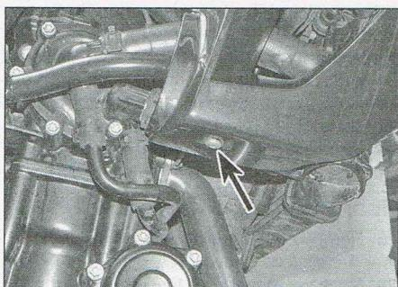
2.14a Undo the screws securing the underside...
