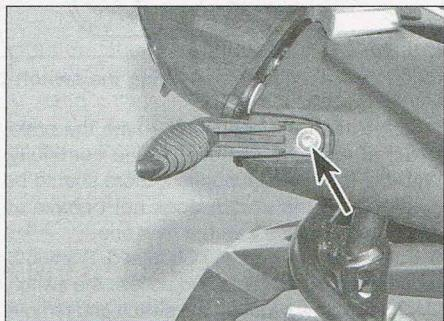
10.11 Screw (arrowed) secures rear turn signal – S, ST, GT and R models
