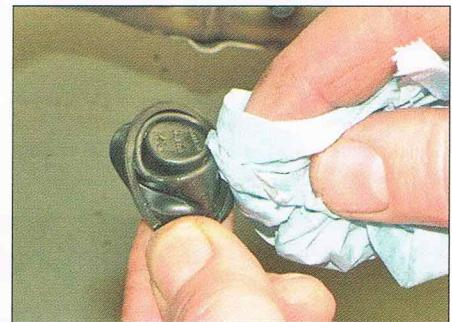
**5** Wipe any moisture off the diaphragm with a clean paper towel. Ensure that the diaphragm is correctly seated, then install the cap and tighten it securely.
