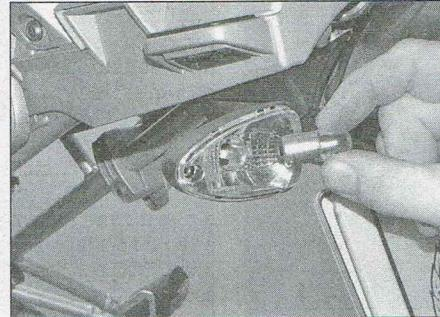
10.3 Push the bulb in and turn it anti-clockwise to remove it
