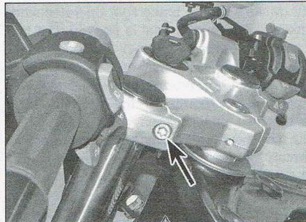
6.8a Loosen the top yoke fork clamp bolts...
