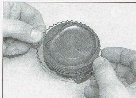
25.4b ...then fit the expander into its groove
