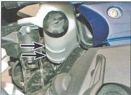
**1** With the motorcycle vertical and level, the coolant level should lie between the MAX and MIN level lines (arrowed) marked on the reservoir. If necessary, remove the right-hand bodywork side panel for access (see Chapter 7).
