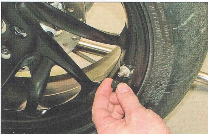
**1** Remove the dust cap from the valve, and do not forget to fit the cap after checking the pressure.
