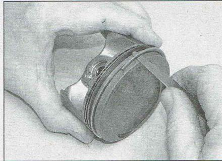
24.5 Using a thin blade to remove the piston rings
