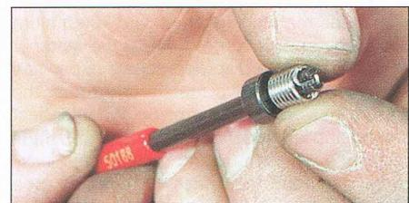
2.28 ... fit insert on the installing tool ...
