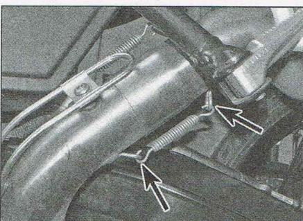
11.7 Align tabs (arrowed) before installing spring
