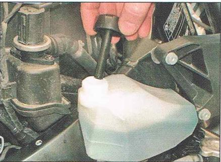
**2** If the coolant level is on or below the MIN line, remove the side panel (see Chapter 7), then unscrew the reservoir filler cap.
