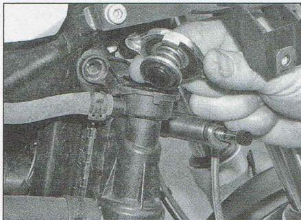
2.4 Remove the radiator pressure cap
