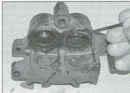
3.17 Remove the old seals carefully to avoid scratching the bores
