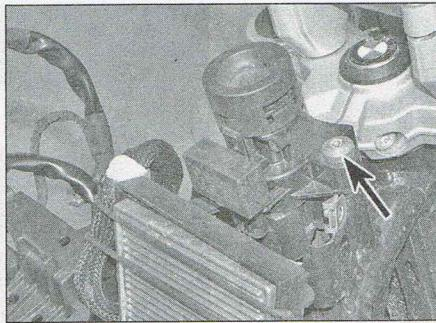
16.10 Ignition switch on GS models is retained by a security Torx screw (arrowed) on each side
