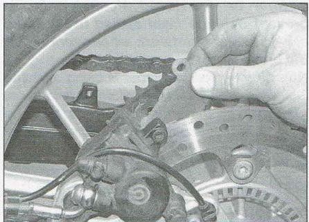
6.3c ...and inner pad out of the caliper – GS and R
