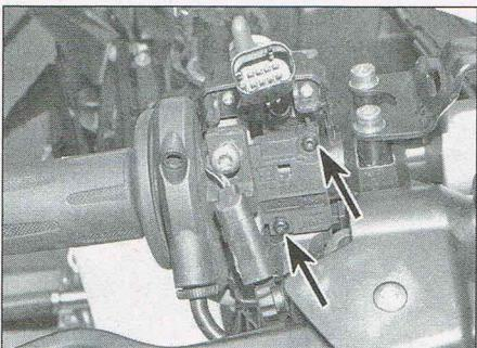
5.5a Undo the screws (arrowed)...
