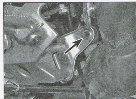
11.22b ...and unscrew the nut on the inside of the bracket
