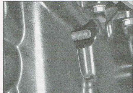
8.3e Installed position of the TDC locating tool
