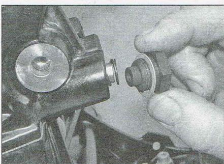
7.2 Note the sealing washer on the cap bolt
