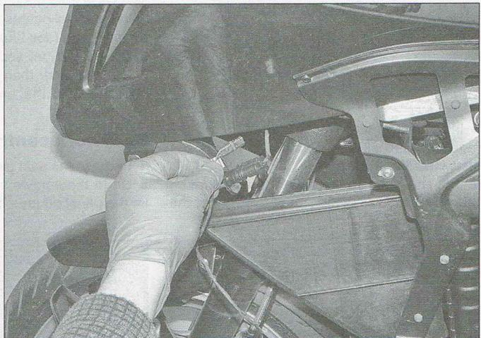
5.14a Disconnect the turn signal wiring connector
