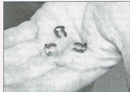
12.4b Examine the clips for damage and corrosion
