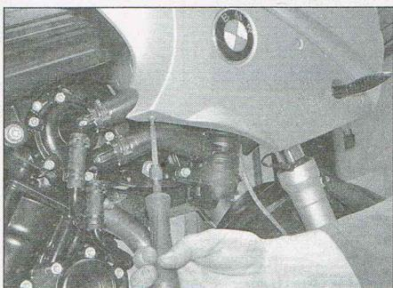
4.9b Undo the screws securing the underside...
