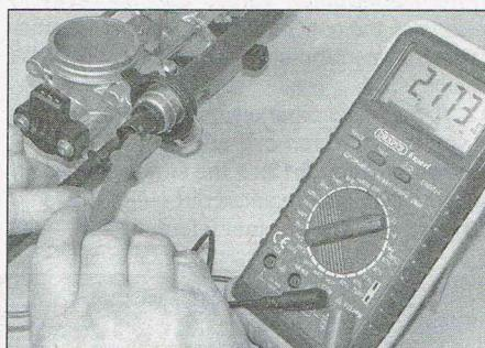
7.3a Measuring the fuel pressure sensor resistance
