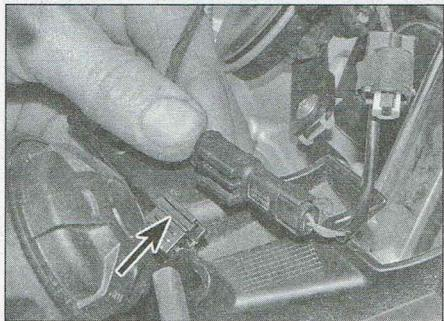
7.6f ...and release the wiring from the clip on the bracket
