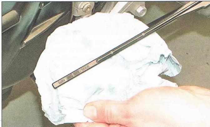
**4** Withdraw the dipstick – the oil level should lie between the MAX and MIN level lines on the dipstick.
