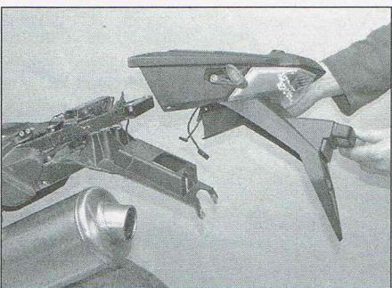
2.28c ...then lift the mudguard assembly off
