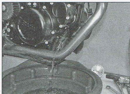
2.6c ...and drain the coolant – S model shown
