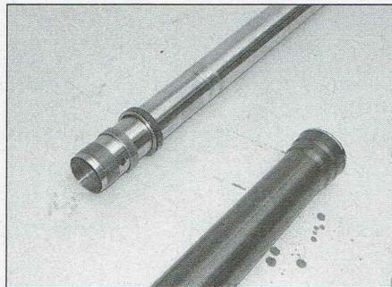
8.54b The oil seal, washer and both bushes will come out on the inner tube
