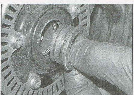
15.7c Note the direction of fitting the axle spacer in the hub left side
