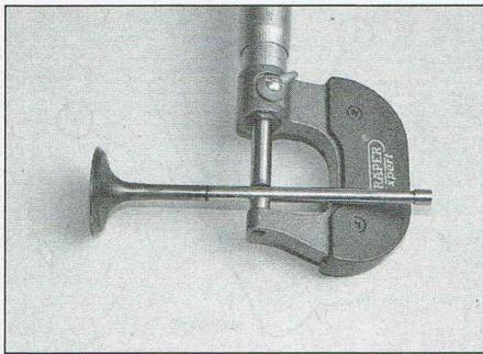
11.25a Measuring valve stem diameter
