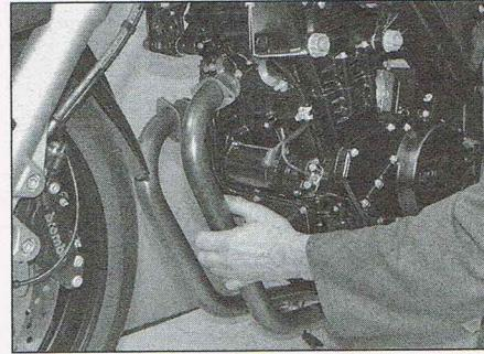
11.24 Detach the downpipes and lift the exhaust off
