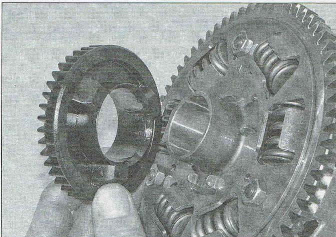
14.20 Note how the tabs on the oil pump drive gear locate
