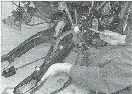
13.48 Installing the swingarm pivot bolt
