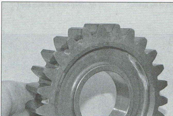
27.10 Inspect the gear teeth for wear and damage
