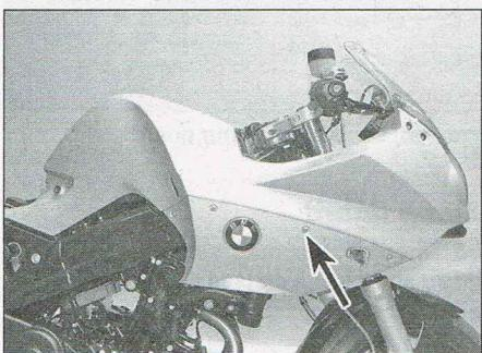
4.9a Undo the screw (arrowed)
