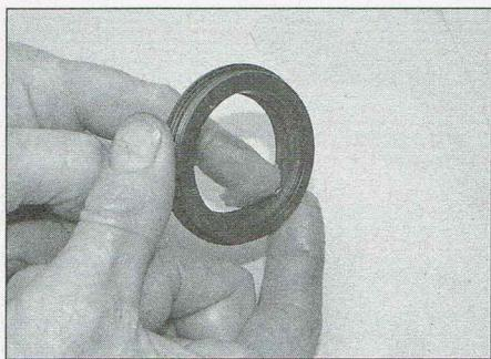
8.26a Fill the groove with grease...
