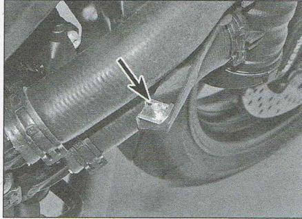
1.4a Ensure all U-clips (arrowed)...
