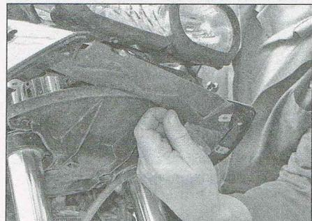
2.13 Remove the joining piece
