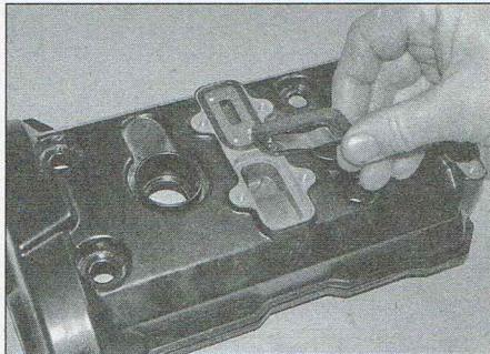
6.14c Note which way round the reed valves are fitted
