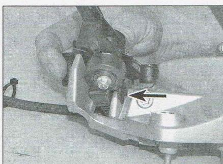
4.11 Note how outside tab (arrowed) on switch locates
