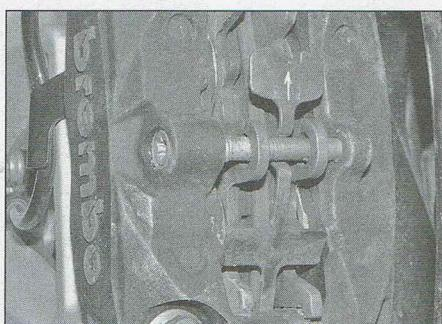
2.23a Pads and spring correctly positioned
