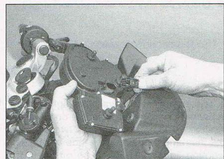
12.5b ...and disconnect the wiring connector
