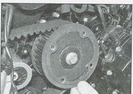
19.5b ...and remove the outer rim of the front pulley
