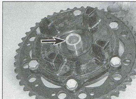
17.37 Drive the bearing and spacer out from the inside
