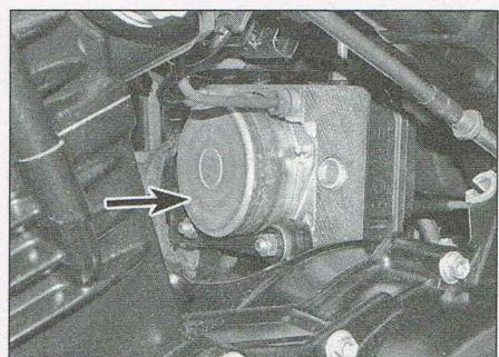
10.2d Location of ABS modulator/control unit (arrowed)
