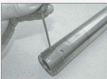
8.16 Remove the bottom bush by levering the ends apart
