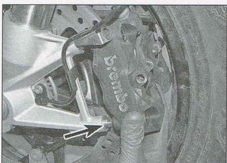
3.43 Refitting the caliper over the disc and dowels (lower dowel arrowed)
