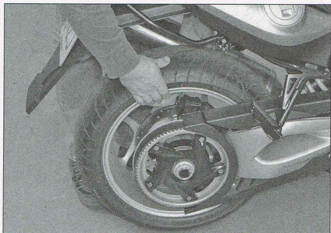
13.11 Checking the rear shock for freeplay
