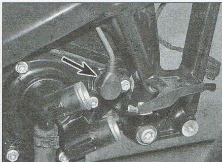
17.9b Location of the camshaft position sensor – S, ST, GT and R models
