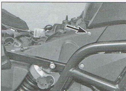
11.3 Undo screws on both sides securing the seat bridge
