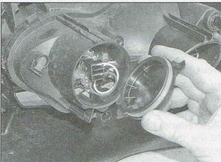
6.20 Remove the high beam bulb cover
