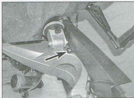
11.8a Upper belt guard fixing screws at rear...
