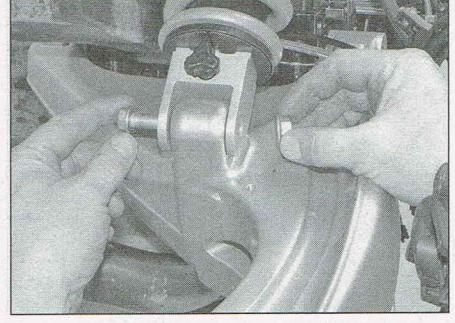
11.14 Nut and bolt secure the lower end of the shock
