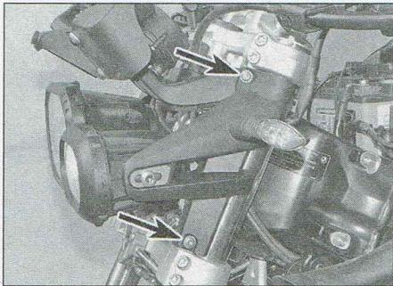
7.6c Undo the screws securing the bracket...
