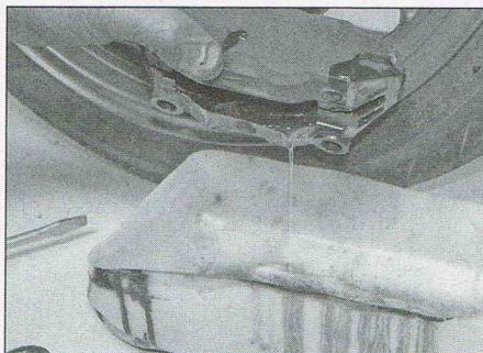
3.30b ...and drain the brake fluid
