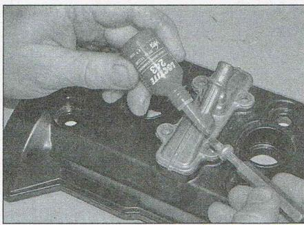
6.17 Apply thread-locking compound to the reed valve cover screws
