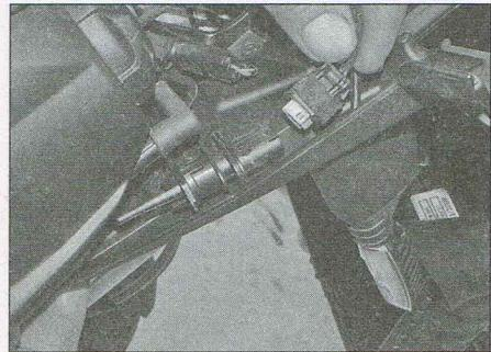
7.6e Disconnect the air temperature sensor wiring connector...
