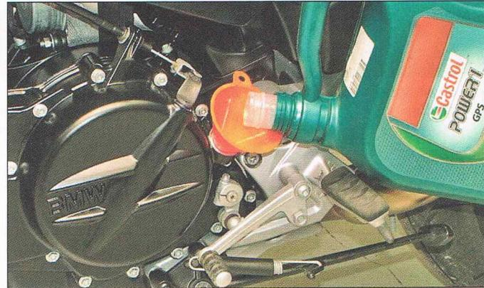
**5** If the level is near, on or below the MIN line, top up with the recommended grade and type of oil so the level lies approximately mid-way between the MAX and MIN lines. **Do not overfill.** If necessary, drain off any excess oil (see Chapter 1). On completion, tighten the filler cap securely. Repeat the warm-up procedure and
