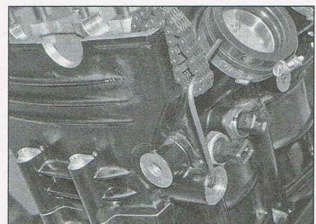
8.6c Secure the cam chain with a length of bent wire
