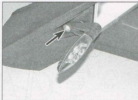
10.10a Screw (arrowed) secures rear turn signal – GS models
