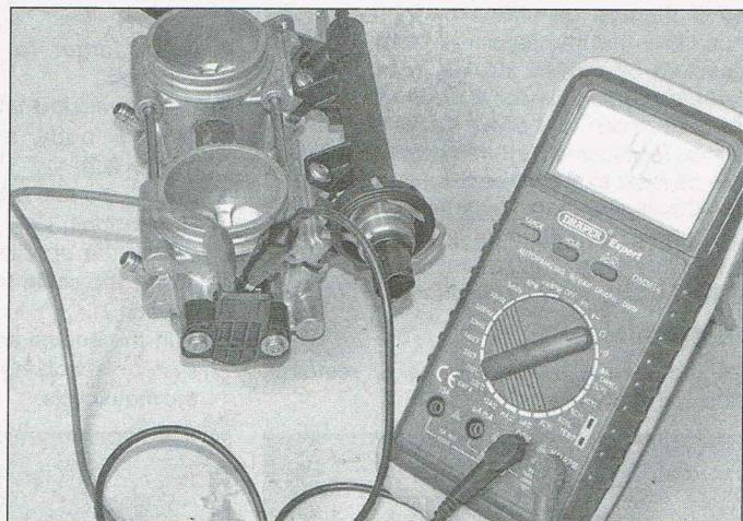
9.18a Measuring the throttle position sensor resistance
