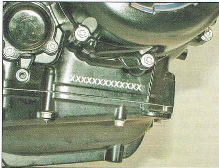
The engine number is stamped into the right crankcase half just below the alternator cover
