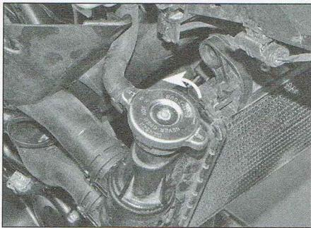
15.8a Turn the radiator cap anti-clockwise...
