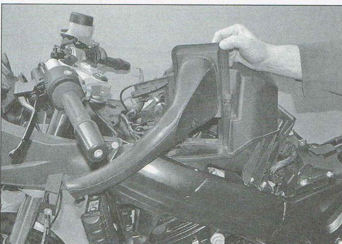
11.3b ...to release the intake pipe...
