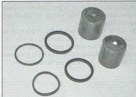
3.20 Match the corresponding seals and pistons before installation
