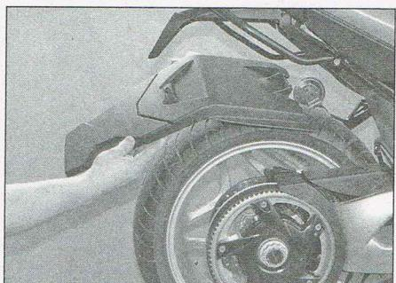
4.35b ...and lift the rear mudguard off
