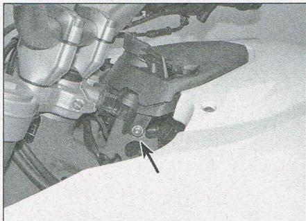
3.3 Undo the screw on both sides
