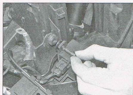
21.2a Release the pins securing the relay...
