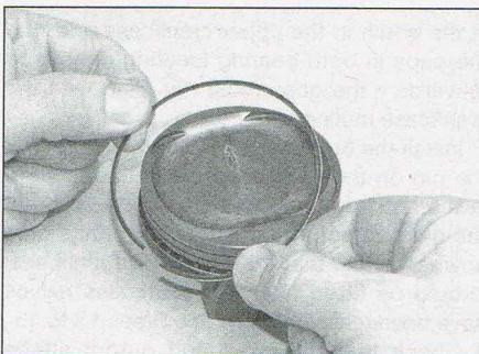
25.6a Fit the second ring onto the piston...
