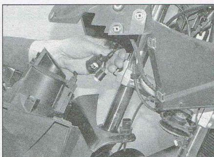
7.18a Disconnect the wiring connectors...
