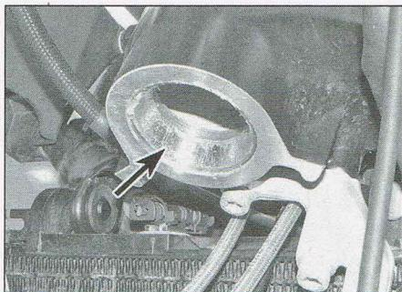
10.3 Check the bearing races for wear and damage
