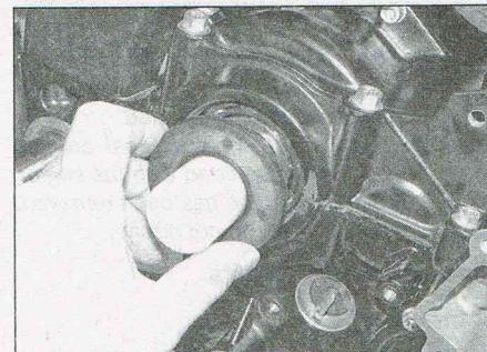
26.14 Lubricate the new seal prior to installation
