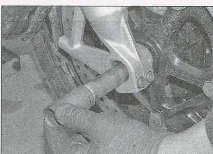
15.7b ...slacken the clamp bolts on the right side and withdraw the axle
