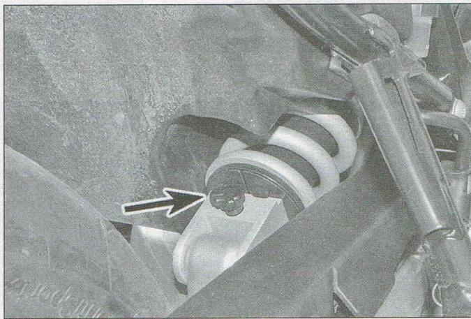
12.5 Spring rebound damping adjuster – S, ST, GT and R models
