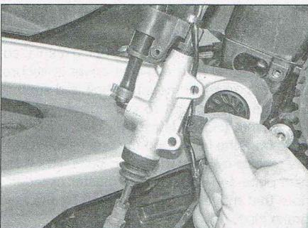
9.13 Unclip the brake light switch wiring
