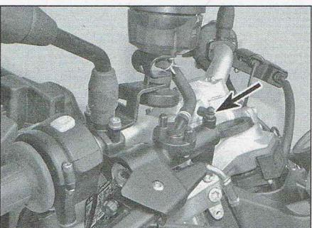
12.4 Master cylinder bleed valve (arrowed)
