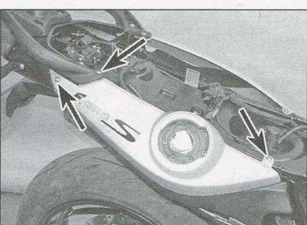
4.31a Undo the screws (arrowed)...
