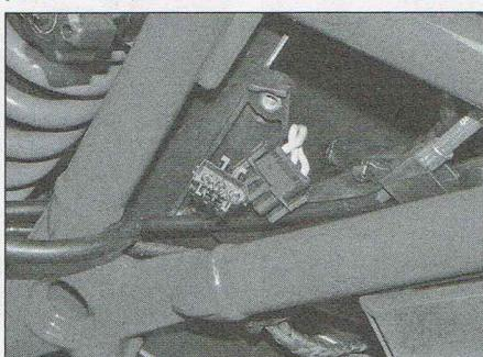
24.4 Disconnect the alternator wiring connector – 2015 F800 GS shown
