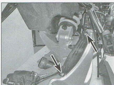
13.10d Screws (arrowed) secure brake hose cover
