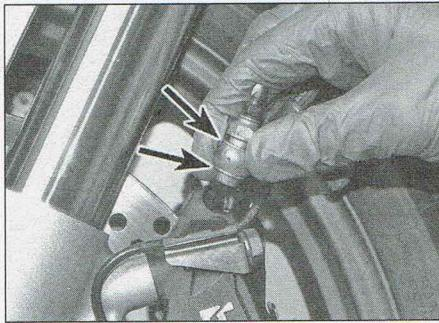
3.44 Use new sealing washers (arrowed) each side of the union
