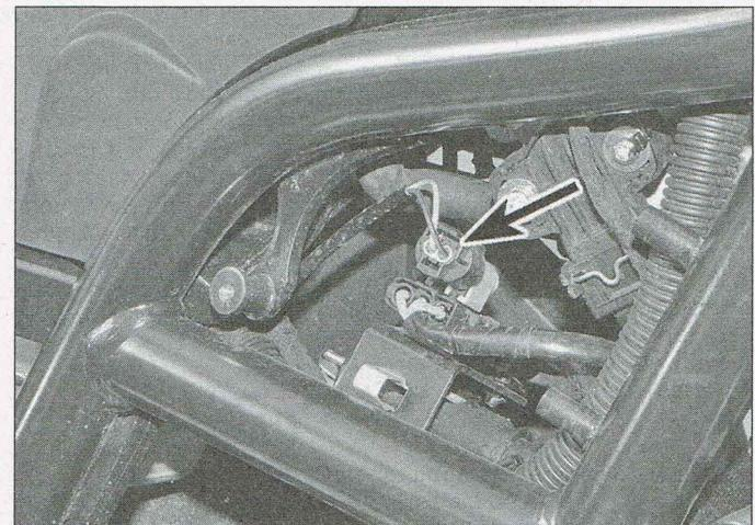
11.7b Disconnect the wiring connector
