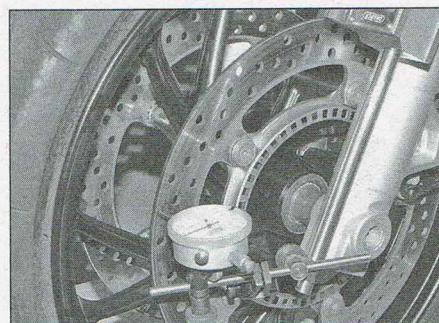
4.3 Set-up for checking disc runout
