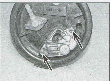
5.10a Undo the screws (arrowed)...
