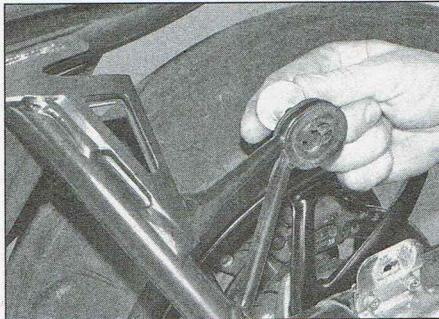
11.12 Inspect the bushing in the silencer mounting bracket
