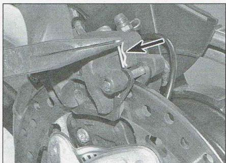
6.5 Pull out the R-clip (arrowed)
