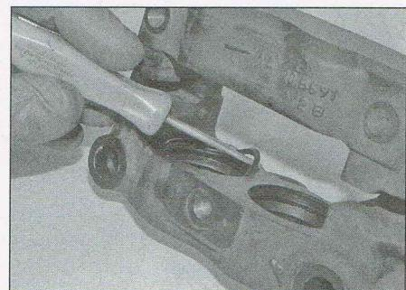
3.32 Pick out the old dust seal and piston seal, but don't scratch the bore surface
