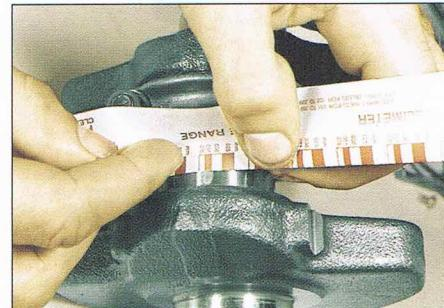
3.16 Measuring the width of the crushed Plastigauge
