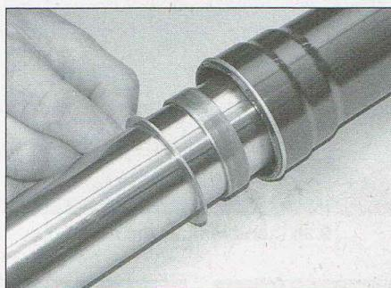
8.71a Slide the lower bush and washer into the bottom of the outer tube...
