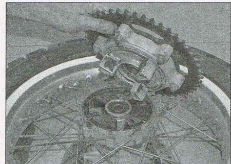
17.43 Lift the sprocket coupling out of the hub
