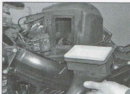
11.7a Fit the filter element into the intake pipe – S, ST, GT and R models
