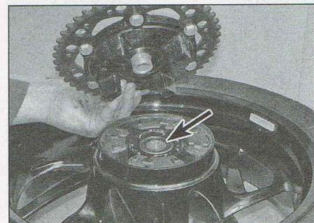
16.11 Check the bearing in the right-hand side of the hub
