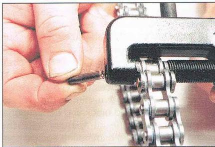
8.2 ... withdraw the pin, remove the tool ...
