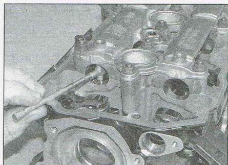
8.18b Measuring the camshaft holder bore diameter
