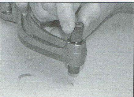
20.9 Checking the balancer rod shaft for freeplay
