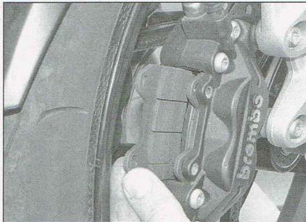
2.6 Draw the pads out of the caliper
