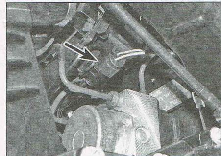
3.4 Location of the sidestand switch wiring connector
