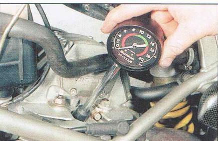
3.20 Using a rubber-cone type cylinder compression gauge
