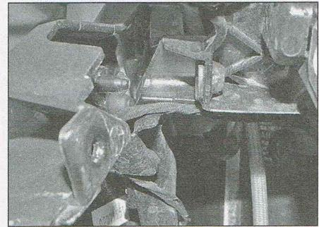
7.12b Peg on inner edge locates in grommet set in the mounting bracket
