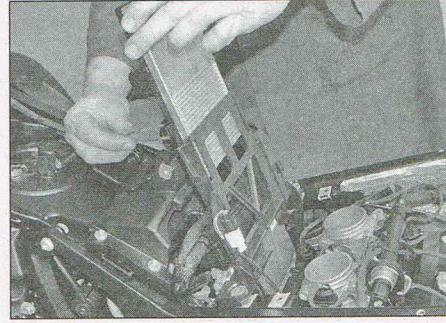
2.8c Lift the ZFE out of its holder – S, ST, GT and R models
