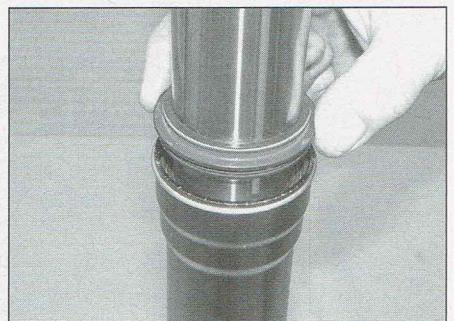
8.74 Press the dust seal into place
