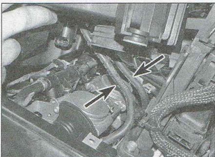
2.18 Disconnect the idle air hoses from the throttle bodies
