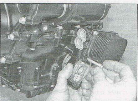
12.7b ...and the flange bolt to the cooler assembly
