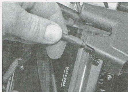
15.3a Pull the cable out from the handlebar bracket...
