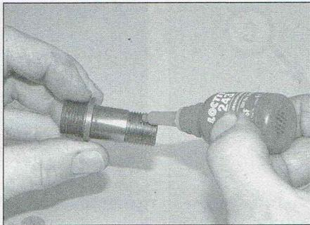
12.11 Thread lock the oil cooler centre bolt
