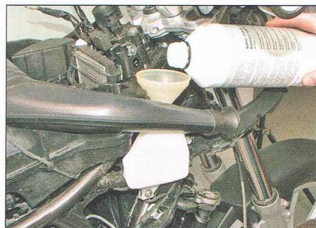
**3** Top the reservoir up with the recommended coolant mixture almost to the MAX level line, using a suitable funnel if required. Fit and tighten the cap. If removed, install the side panel.
