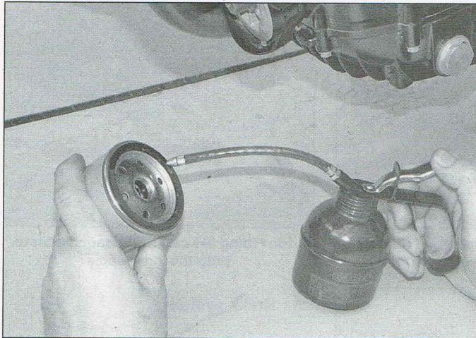
3.7a Lubricate the filter seal...
