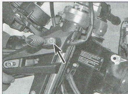
10.8 Front turn signal is secured by screw (arrowed)
