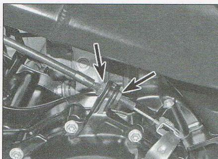
4.4 Loosen the locknuts (arrowed) on the adjuster
