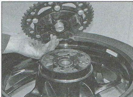
20.2a Lift out the sprocket coupling...
