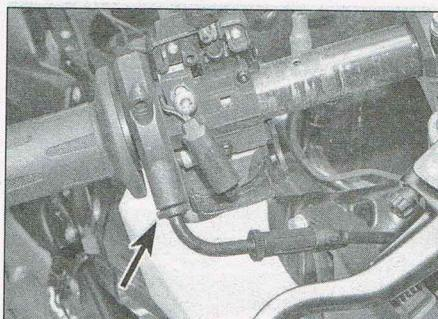
8.6a Unscrew the retaining ring...
