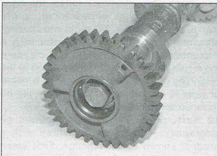
8.21 Inspect the pump drive gear teeth. Retaining bolt has left-hand thread
