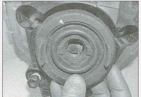
6.15a Pull the dust cover off the back of the headlight...
