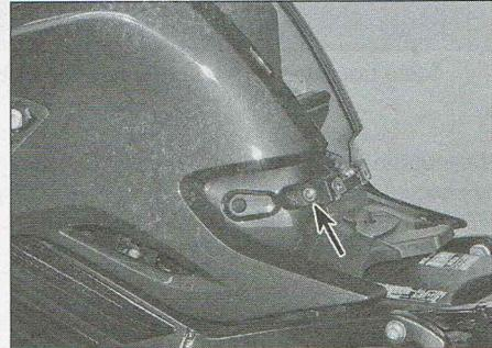
5.21 Undo the screw (arrowed)
