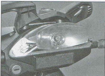
8.2 Push the bulb in and turn it anti-clockwise
