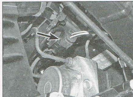
17.2 Location of the sidestand switch wiring connector
