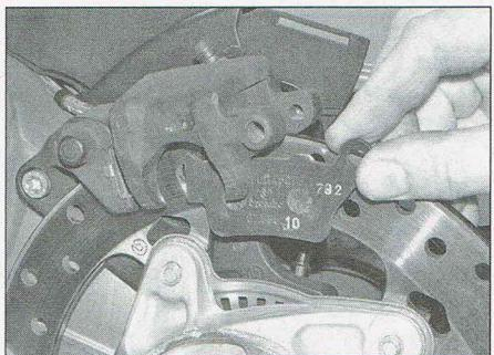
6.6b ...and outer pads out of the caliper – S, ST and GT
