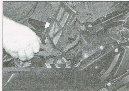
16.6a Release the tie securing the ZFE wiring...
