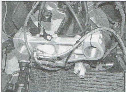
9.19 Ensure all wiring and hoses are correctly routed
