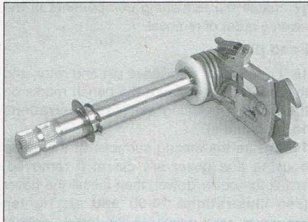
17.5c Check the gearchange shaft for wear and damage
