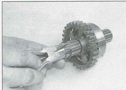
27.32a Remove the circlip...
