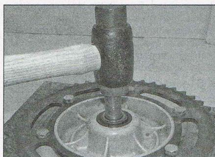
17.44a Drive the inner spacer out of the outer spacer...
