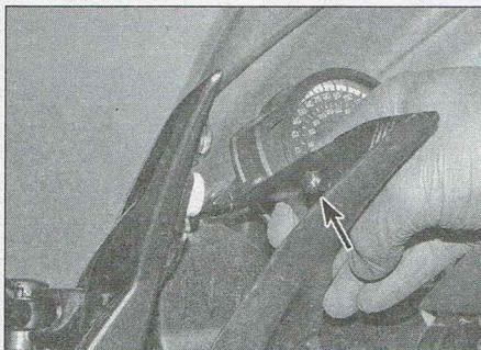
5.8 Pull the peg (arrowed) out from the grommet
