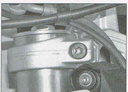
6.8b Fork top bolt aligned with inner raised section of top yoke – 2015-on R models
