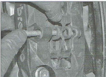
2.8a Unscrew the pad pin and remove the spring...
