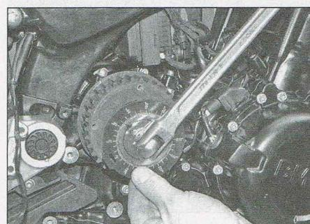
19.24 Using a torque angle gauge to tighten the pulley bolt
