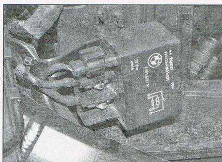
21.1 Starter motor relay – S model shown
