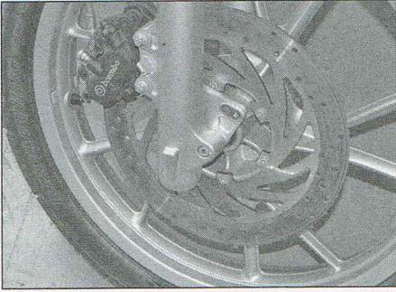
4.1 Inspect the disc for score marks and damage
