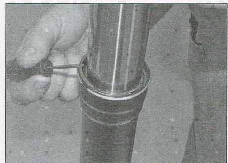
8.53 Ease out the oil seal retaining clip
