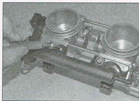
10.9 Thread-lock the fuel rail screws
