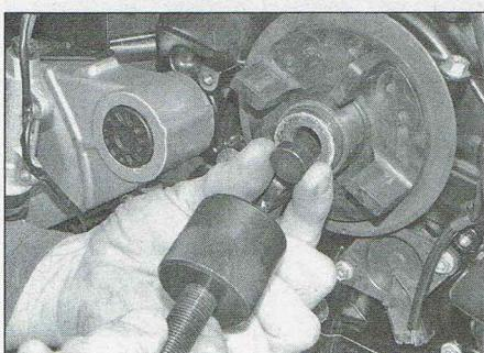
19.21 Installing the blanking piece and puller
