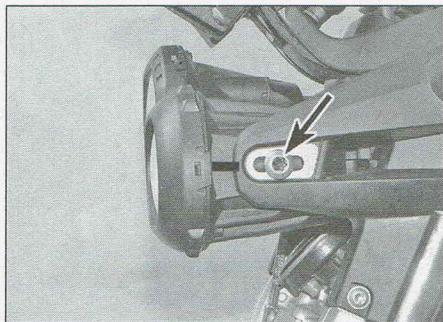
7.3 Note alignment of the headlight unit, then undo the mounting screws (arrowed)
