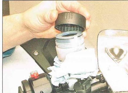
**2** To top-up, press the locking tabs in and unscrew the cap.
