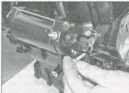
22.4 Undo the bolts securing the starter motor
