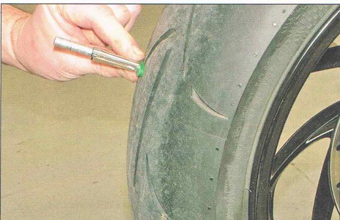
**3** Measure tread depth at the centre of the tyre using a depth gauge.
