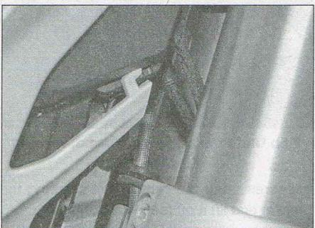
7.9c ...and disengage the hook
