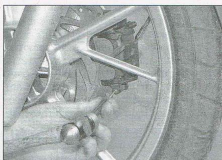
2.17 Drive the pad pin through with a suitable punch
