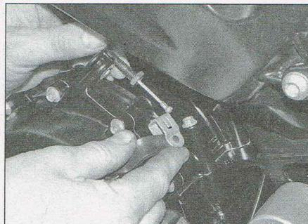
15.2b Slip the cable out through the slot in the bracket
