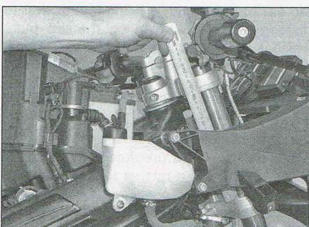
6.7 Measuring fork tube installation – S and ST models
