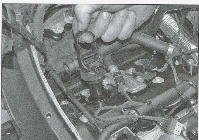
12.6c Using the ignition coil puller
