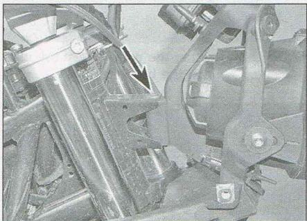
7.5c ...and the bracket centre mounting bolt
