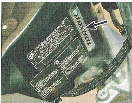
Frame number and VIN plate on S, ST, GT and R models
