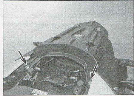
3.17 Screws (arrowed) secure top cover
