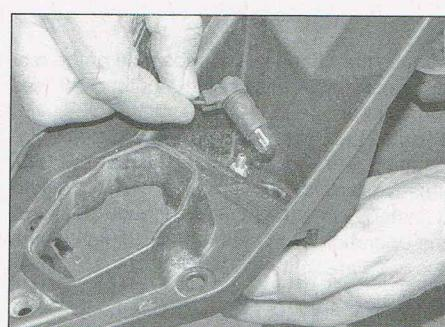
8.8 Ease the bulbholder out from the light unit
