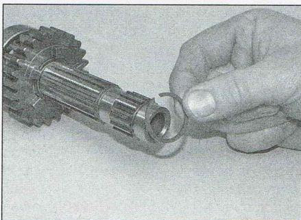
27.18a Ensure the new circlip...
