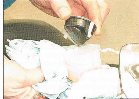
**3** Remove the diaphragm plate and diaphragm.
