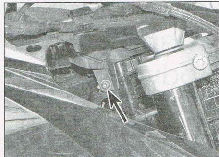
2.5 Undo screw on both sides of ignition switch panel
