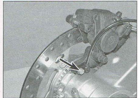
10.10c Undo the bolt (arrowed)...
