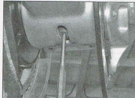
19.4b Use a punch to slacken the drive belt
