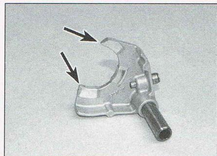
28.7 Inspect the selector forks for wear or damage
