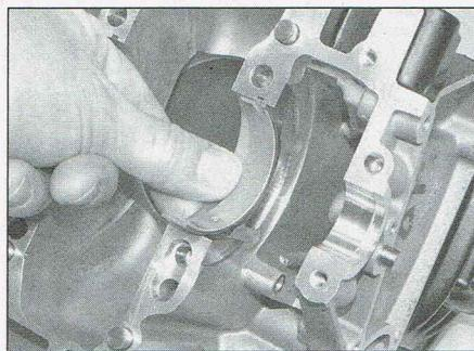
23.10 Remove the shells by carefully pushing them to one side
