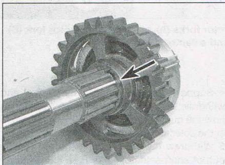
27.38 Ensure the 2nd gear circlip (arrowed) is correctly installed
